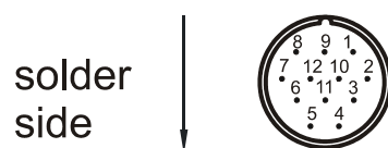
Fig. 21: RC series mating connector of the resolver (internal thread M23)
