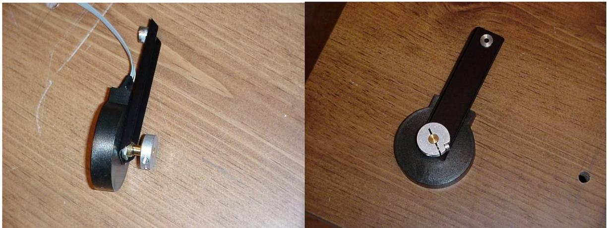
Figure 5-6: Pendubot Link/Encoder Assembly
