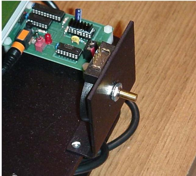
**Figure 5-4: US Digital Encoder Attached to Front Bracket**
