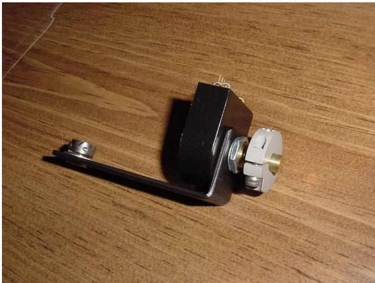
**Figure 5-12: Furuta Link/Encoder Assembly**
