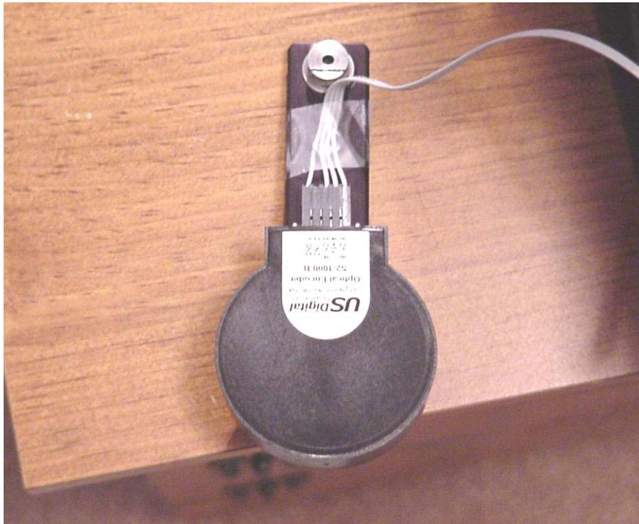
**Figure 5-15: Taping the Encoder Cable to Pendubot Link-1**
