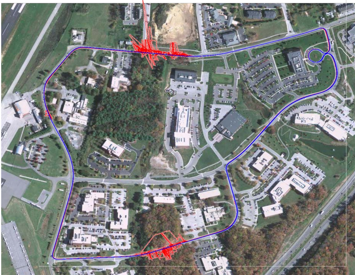
Figure 1: PinPoint™ Filter Output vs. Raw GPS Data
