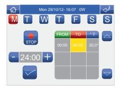
NOTE: daily climate control programming must refer to the whole 24-hour cycle; any hours not programmed by the user will be set by the system automatically.
