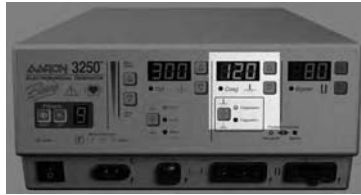
Figure 2 – 4 Controls for the Coag mode
