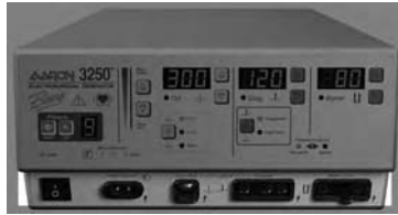
Figure 2 – 7 Location of the unit power switch and front panel receptacles
