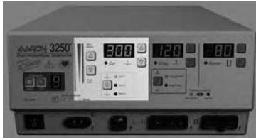
Figure 2 – 3 Controls for the Cut and Blend modes
