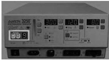
Figure 2 – 2 Controls for setting and recalling presets
