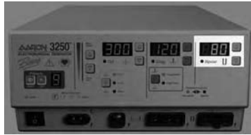
Figure 2 – 5 Controls for the Bipolar mode
