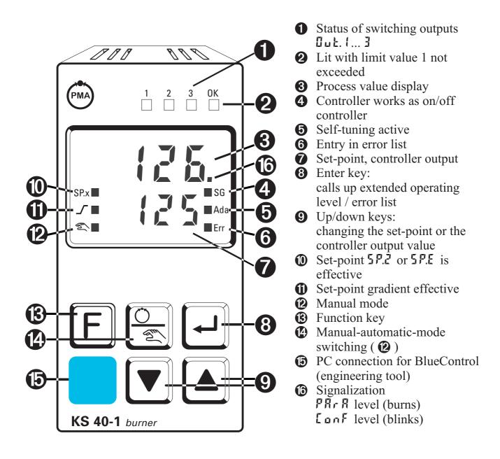
In the upper display line, the process value is <u>always</u> displayed. At parameter, configuration, calibration as well as extended operating level, the bottom display line changes cyclically between parameter name and parameter value.
