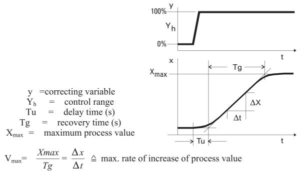
The control parameters can be determined from the values calculated for delay time  $T_u$ , maximum rate of increase  $v_{max}$ , control range  $X_h$  and characteristic K according to the **formulas** given below. Increase Xp, if line-out to the set-point oscillates.
