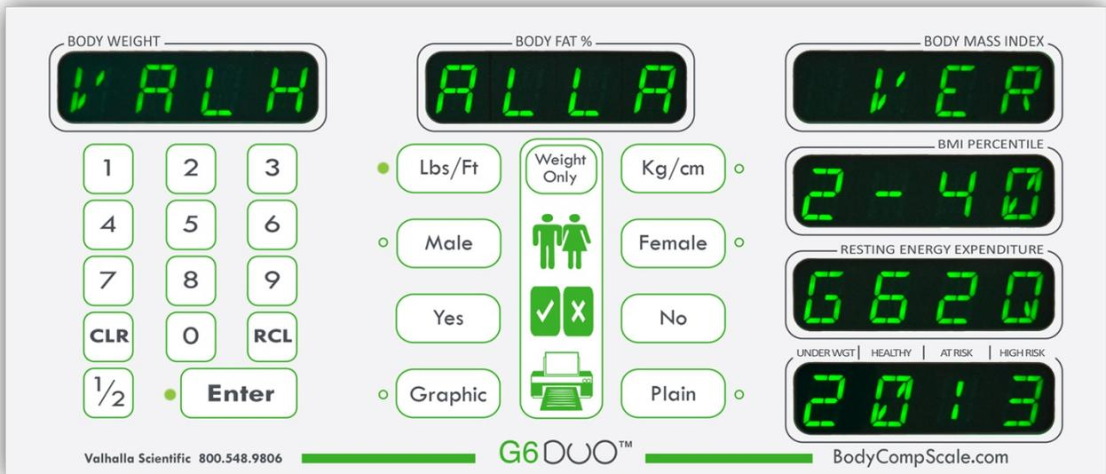
The startup will be followed by a synchronization countdown. Once the display goes blank, the scale is ready to be used.
