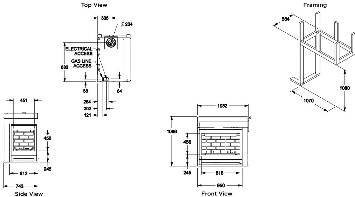
Dimensions above are in millimeters and for reference only. We recommend measuring individual units at installation. Assumes the use of 13mm gyprock.
