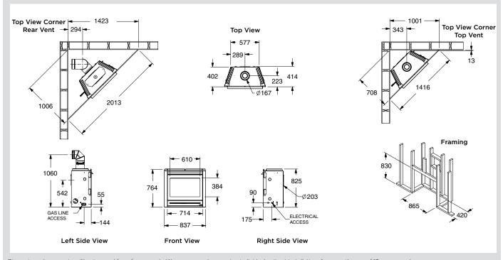
Dimensions above are in millimeters and for reference only. We recommend measuring individual units at installation. Assumes the use of 13mm gyprock.
