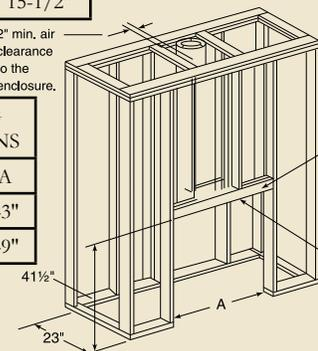
Note: Fireplace header cannot be positioned until after the fireplace assembly is in place.
