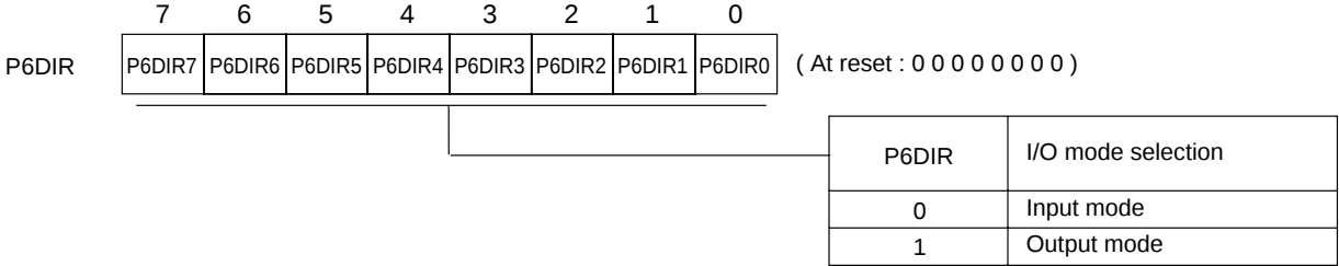
Port 6 direction control register (P6DIR : x'03F36', R/W)
