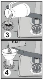
compartment gets filled with water. Therefore, put the softener salt prior to starting your machine.
