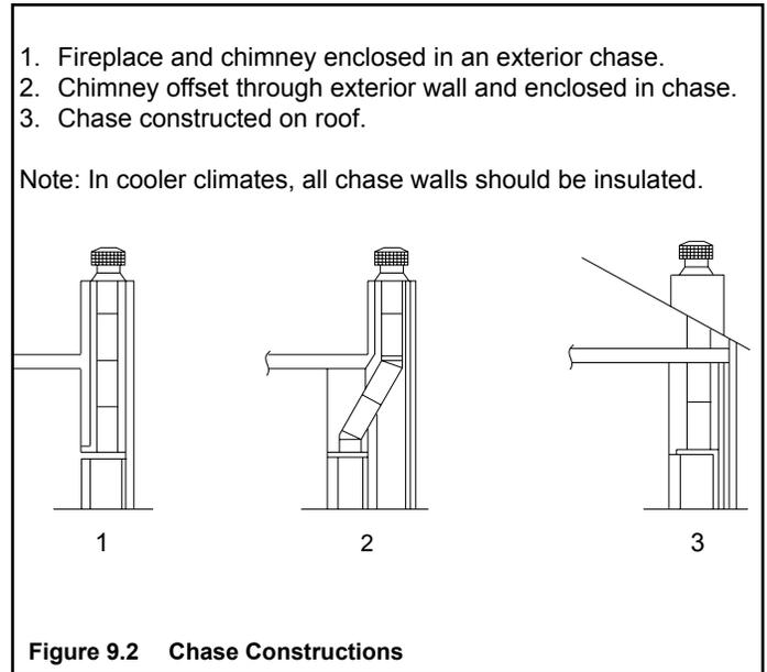
**WARNING!** You must install false ceilings and ceiling firestops at each floor of the chase or every 10 ft (3.05 m) to control spread of fire.
