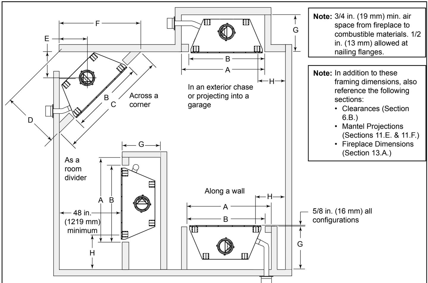
**Note:** Measurements are FRAMING dimensions only and do not include drywall either in the cavity or on the interior walls.
