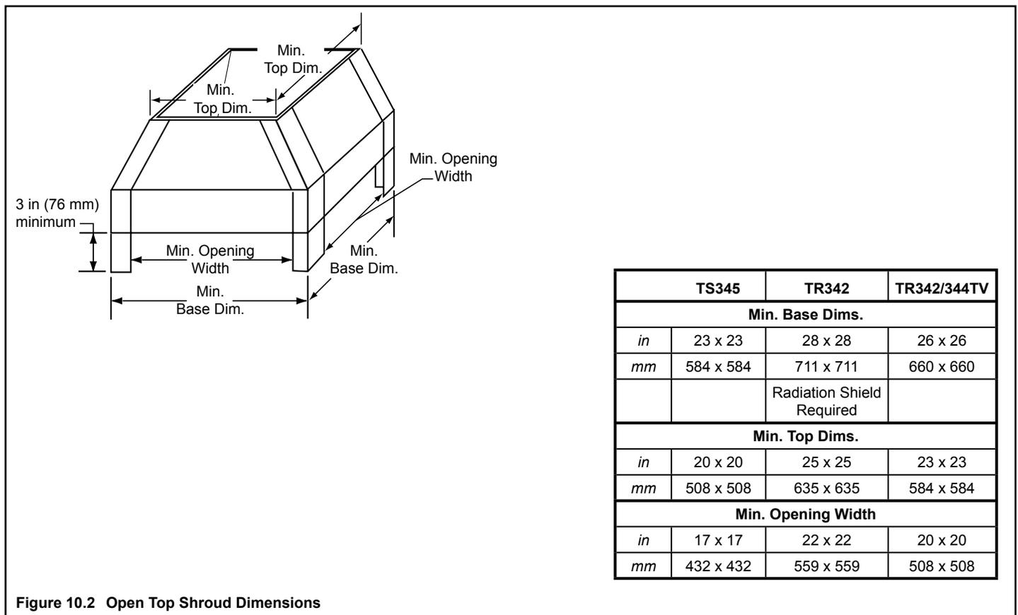
Figure 10.2 Open Top Shroud Dimensions
