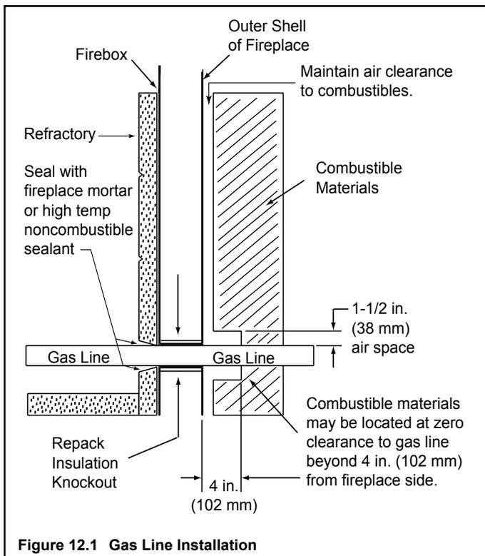
Figure 12.1 Gas Line Installation
