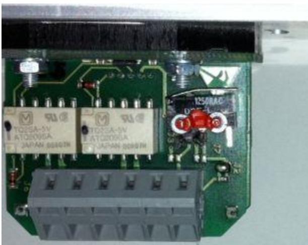
Figure 4: This picture shows a bent switch and will lead into malfunction. Adjust it as shown in figure 1.
