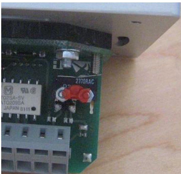
Figure 1: The stud bolt of the front panel operates the sabotage switch – the sabotage loop is closed.
