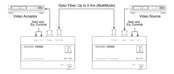
Figure 3: A typical application using the 611T/611R system
