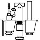
8. Push in control knob all the way and hold in. Immediately depress red or black piezo button. It may require several depressions of the red or black piezo button until PILOT lights. If PILOT light does not light after 10 seconds, return to step 3. Continue to hold the control knob in for about one minute after the pilot is lit. Release knob and it will pop back out. Pilot should remain lit. If it goes out, repeat steps 3 through 6.
