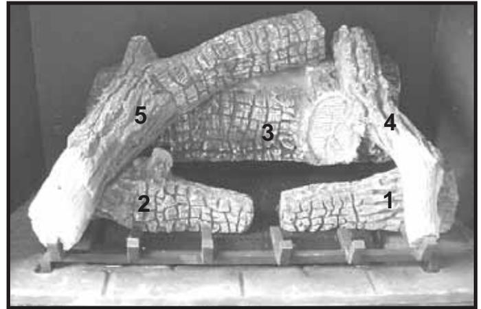
**STEP 6:** (SRV2057-724): Notch in left end of Log 5 will interlock with front left corner of grate. Rest right end of log so that it engages tab on log 3. Log 2 may need to shift to right slightly.
