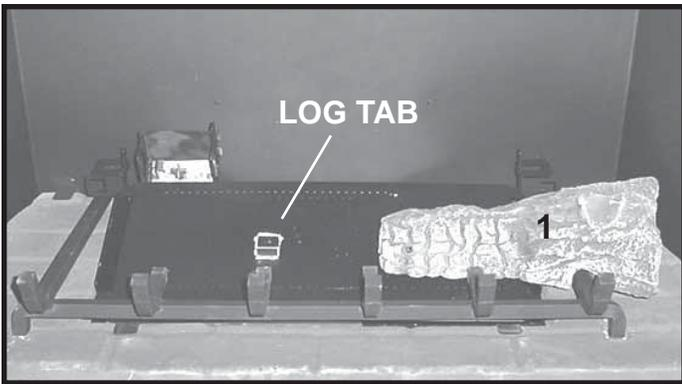
**STEP 2:** Log #1 (SRV2057-720): Place log 1 so that the bottom right notch on log rests on far right grate tine. The bottom left notch on log #1 must mate over the log tab on the burner face.
