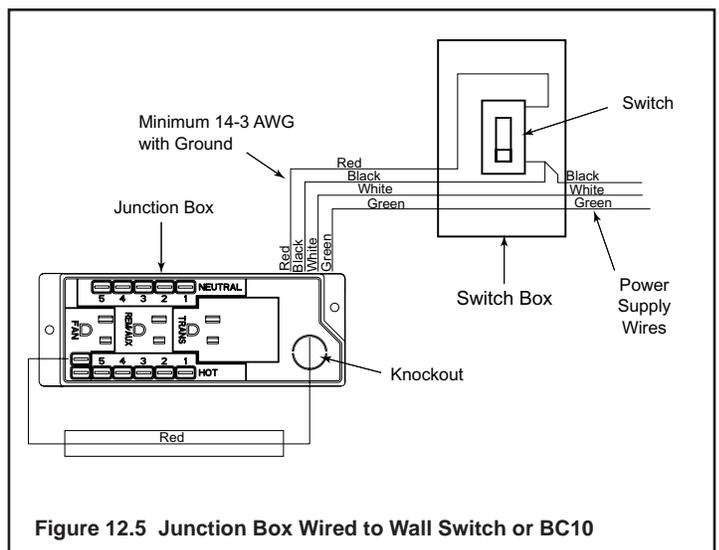
Figure 12.5 Junction Box Wired to Wall Switch or BC10
