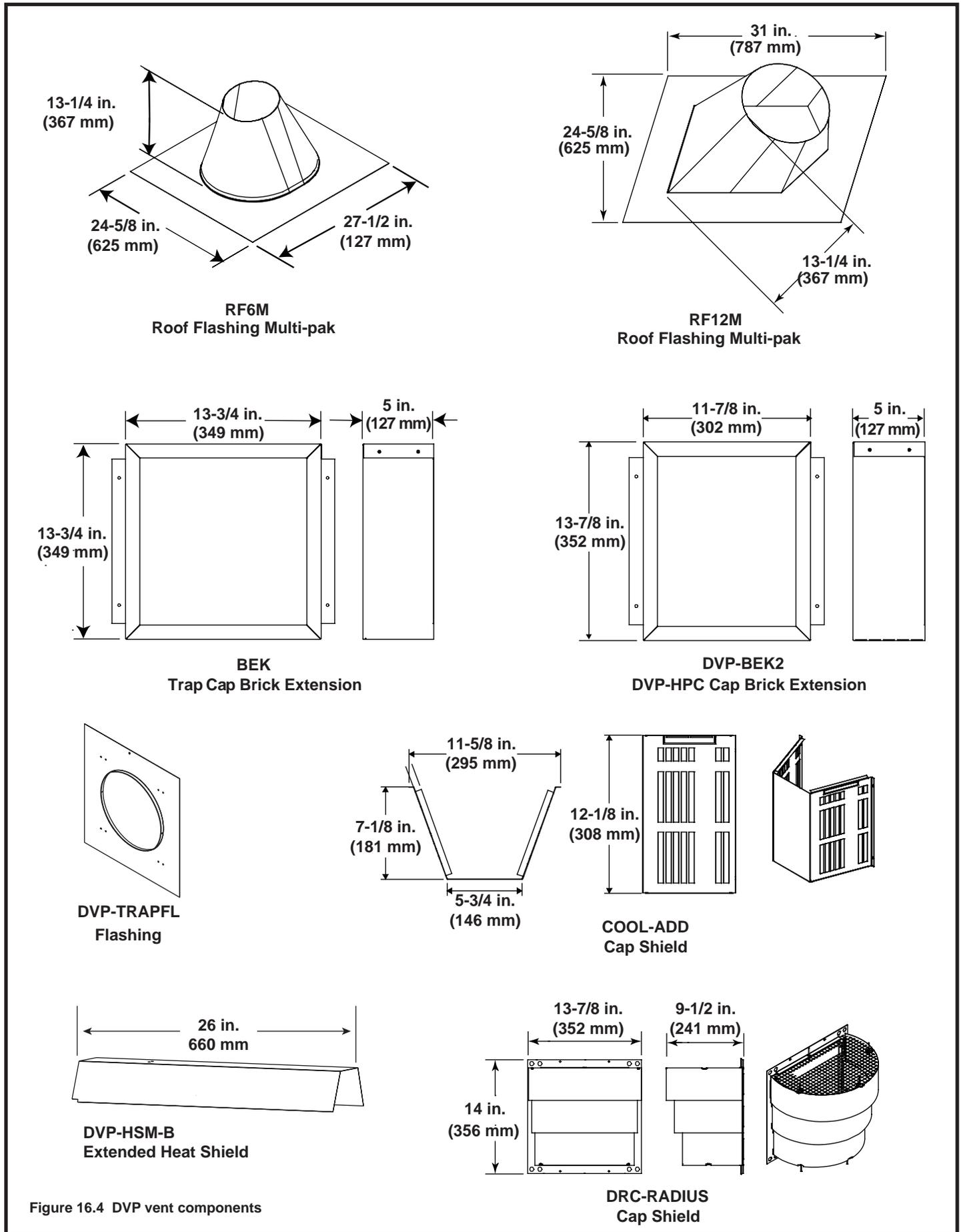
Figure 16.4 DVP vent components
