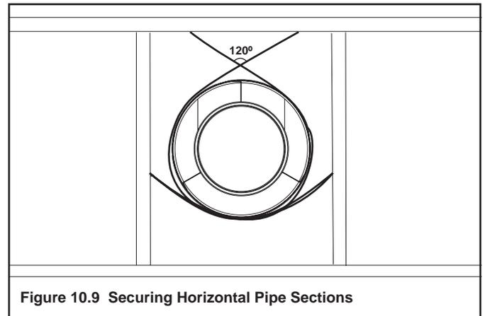
Figure 10.9 Securing Horizontal Pipe Sections
