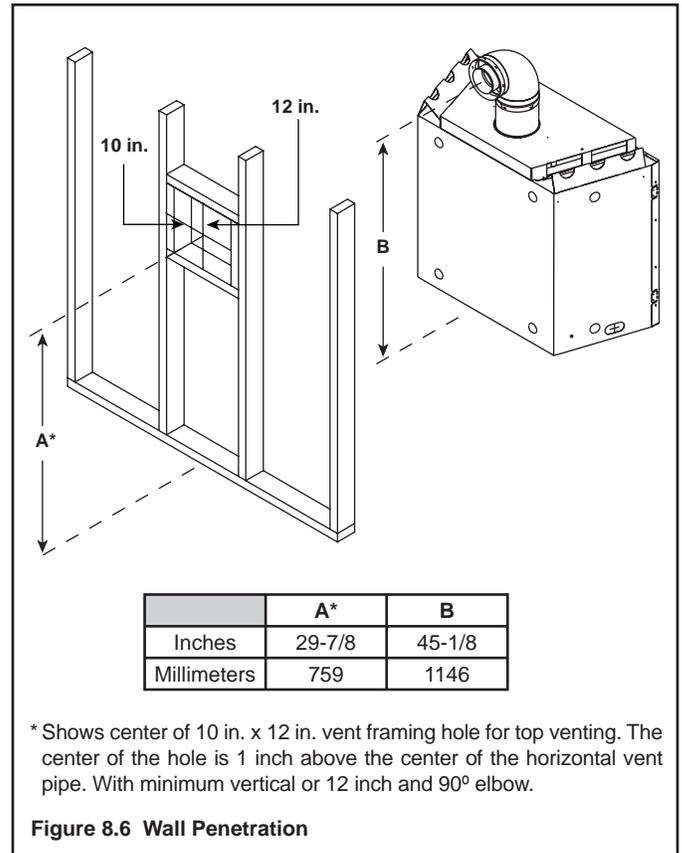
\* Shows center of 10 in. x 12 in. vent framing hole for top venting. The center of the hole is 1 inch above the center of the horizontal vent pipe. With minimum vertical or 12 inch and 90° elbow.
