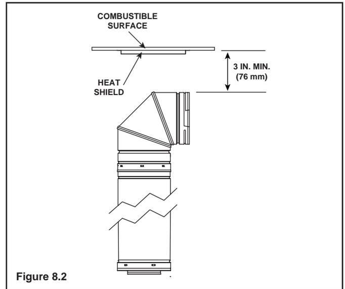
Fasten the shield in place using the four pilot holes provided in the part.
