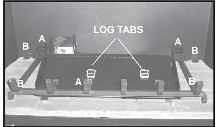
**STEP 1:** Remove metal grate supports (A) and refractory tabs (B) by using a back and forth motion until the tabs break free. Metal tabs and supports are needed for shipping only. After removing the tabs and supports, the grate should fully rest on the base refractory.
