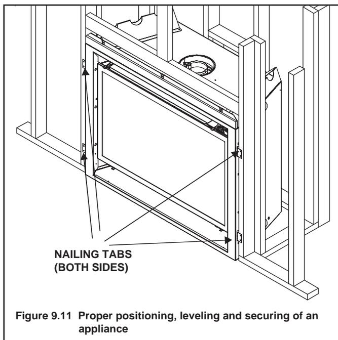
Figure 9.11 Proper positioning, leveling and securing of an appliance
