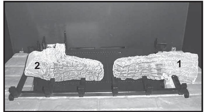
**STEP 3:** (SRV2057-721): Place log 2, nose to nose with log 1. The bottom notch on log #2 must mate over the log tab on the burner face.
