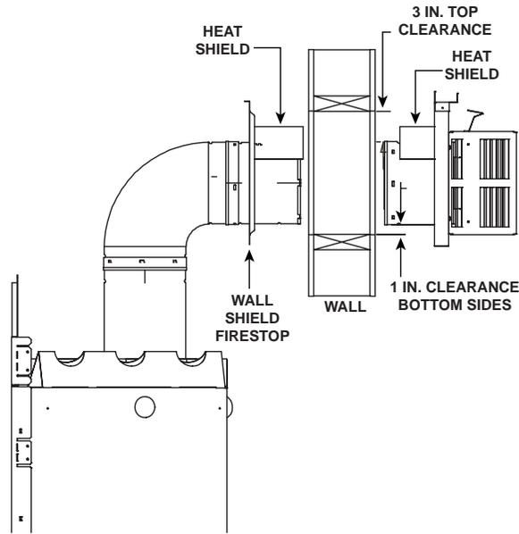
Figure 8.5 Horizontal Venting Clearances to Combustible Materials
