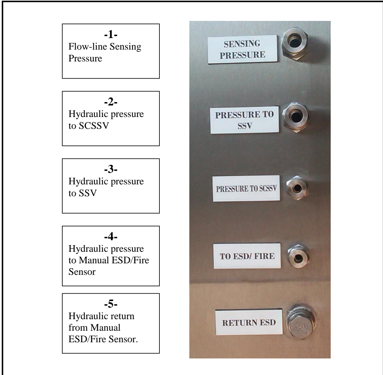
Fig. 4 – Rear view, hydraulic lines connections.
