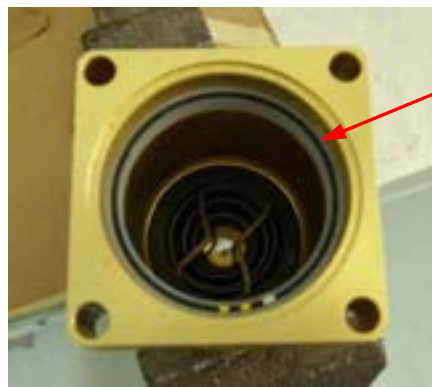
Piston Seal – install with the o-ring or spring facing up
