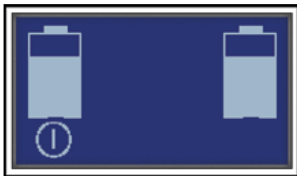
Figure 6. Typical startup screen showing 2 batteries, each 3/4 charged.
