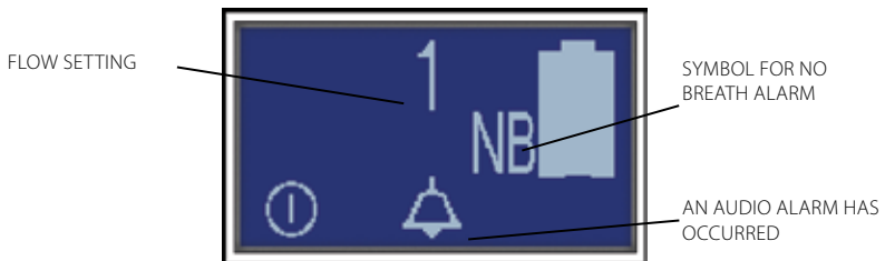
Figure 18. Example of an alarm screen. If the device does not detect breathing for 30 seconds or more, it will sound the NB alarm and show this typical display with the NB alarm symbol (NB = No Breath). The alarm symbol (bell) shows the audio alarm is on. To silence the audio alarm, press the alarm symbol. For a complete list of alarms, see page 19.
