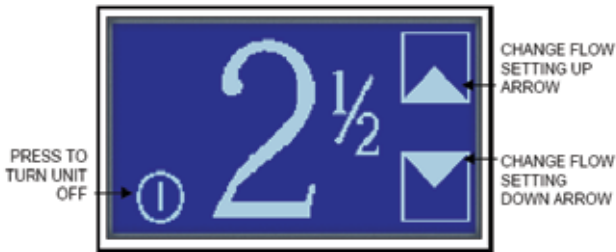
Figure 17. To change the flow setting, touch the setting number; here it is 2 1/2. This causes the up and down arrows to appear. To increase the flow setting, press the up arrow on the right until you reach your prescribed setting. To decrease your flow setting, press the down arrow. The flow setting arrows disappear when you touch the number again or 5 seconds after you touch the screen.
