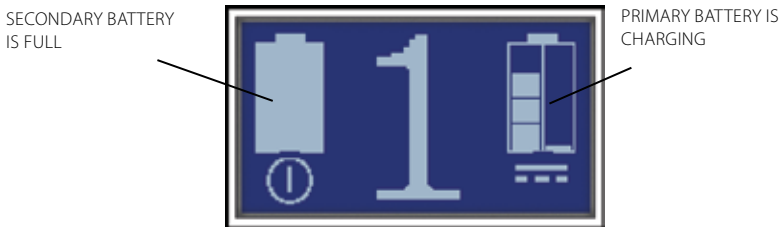
Figure 15. This display shows that two batteries are inserted. It also shows that the unit is connected to a power source. The secondary (left) battery is fully charged. The primary (right) battery is nearly empty and charging.
