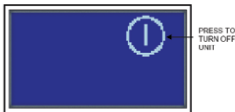
Figure 20. Typical display after touching the On/Off symbol on the previous screen to turn off the device. You must press this symbol again, on this screen, to turn off this device. If this symbol is not pressed within 5 seconds, the previous screen will reappear and the device will remain on.
