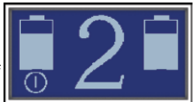
Figure 9. Touch the number to change the flow setting
