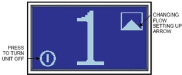
Figure 16. To change the flow setting, touch the setting number (Here, it is the number 1). This causes the up flow change arrow to appear. To increase the flow setting, press the up arrow until you reach your prescribed setting. The flow setting arrow disappears 5 seconds after you touch it. For another example of the flow change arrows, see the next figure.
