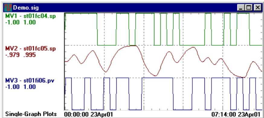
then the correlation curves should be updated. To do this select Build>Step Test Signals from the main menu and remember to use the “Correlation Only” option. (If this is not done, the modified data will be overwritten with a new signal.)
