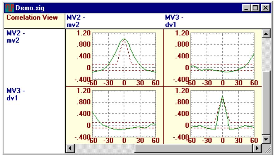
While design goals for both the power spectrum and the auto and cross-correlation functions are attained for unaltered signals, data modification may result in substantial performance deterioration. Note, for modified signals good correlation results do not necessarily imply a good power spectrum. In particular, filtering can have a drastic negative affect on the power spectrum (which as yet is not available). If filtering signals USER BEWARE.
