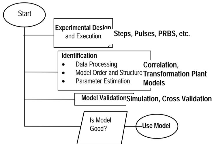
This document is concerned only with the experimental design portion of the above diagram. Identification and model validation techniques are described in detail in the APC Identifier User's Guide.
