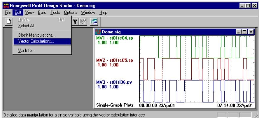
Either the “Block Manipulation” or “Vector Calculation” mode can be used to modify the data. For a full description of these editing functions see the APC Identifier User’s Manual. After editing data remember to always check the correlation curves for the modified data. For example if “MV2” is filtered as shown below,
