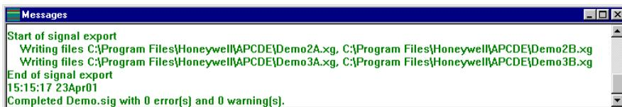
Notice that there are actually four files generated for this example. There is an A and B file created for each signal. Due to a parameter list read limitation on the LCN, export files are limited to 500 elements.
