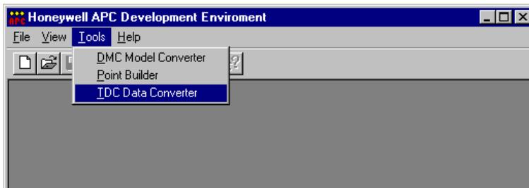
This action brings up the TDC Data Converter dialog box. If the TDC Data Converter selection is "grayed out" under the Tools menu, then it probably has not been installed correctly. Be sure to install the TDC Data Converter in the same directory as the APCDE.
