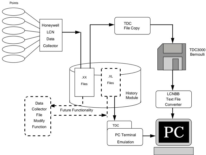
Figure 1--Block Diagram of Data Collector Information Flow
