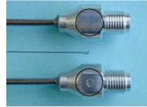
• Sniffer probe equipped with a  $\varnothing$  0.30 mm needle has no mark or is marked "0".
