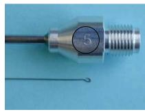
• Sniffer probe equipped with a Ø 0.35 mm needle is marked "5".
