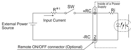
Fig.7.1 Example of using a remote ON/OFF circuit
