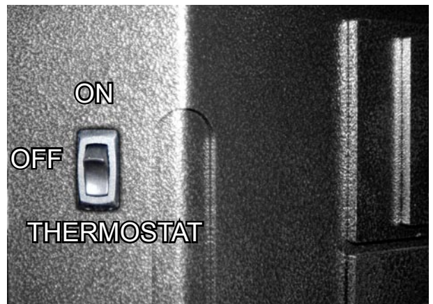
UP - ON MIDDLE - OFF DOWN - THERMOSTAT
