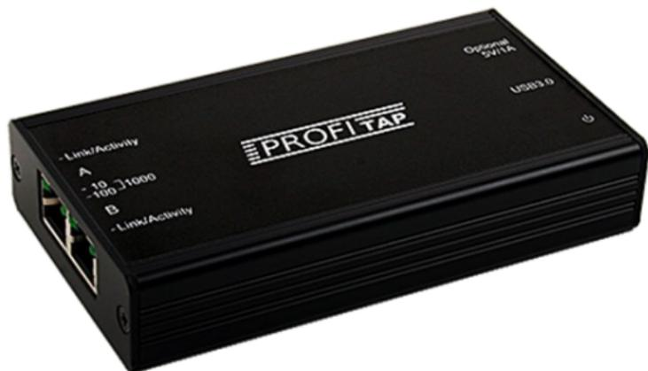
The PROFISHARK is a handheld, Plug and Play device dedicated to inline gigabit monitoring. It facilitates in-field traffic capture and troubleshooting. The PROFISHARK is equivalent to a 10/100/1G aggregator TAP and a 2 Gbit/s NIC. All-in-one in a pocket-sized box, the only additional hardware required being a laptop with a free USB 3.0 port.
