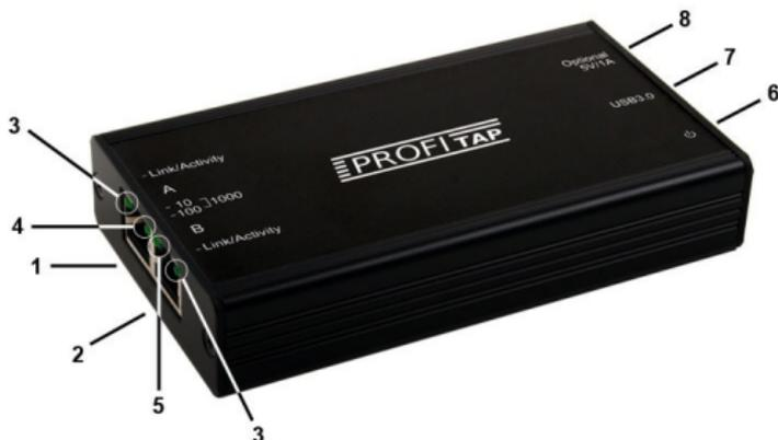
1. Port A (RJ45) connected to the network
