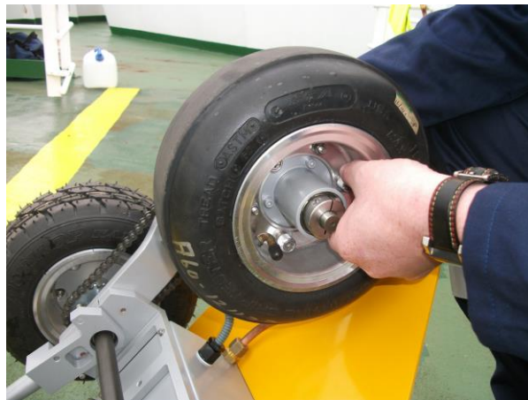
Fig 5: Drive wheel fitted with 3 nuts.
