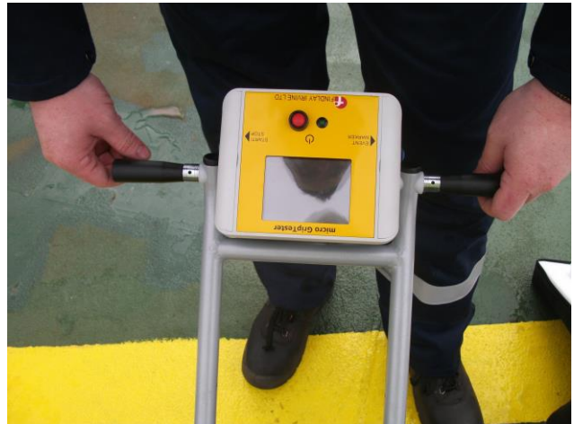
Fig 11: Push handles in survey position
