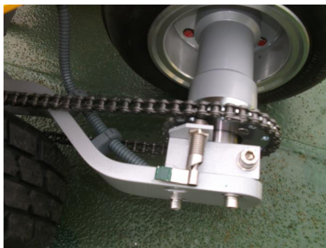
Fig 17: Locking mechanism, rotated to show Green.
