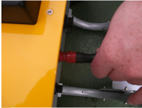
Fig 9: Line up the two markers before fitting.
