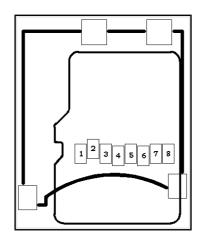
Notice that the pad numeration is written at the bottom of STM32-E407 under the microSD card connector.
