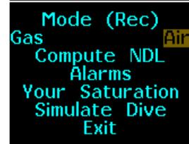
Then tap Up to increase the oxygen % to your desired value. The gas will switch from "Air" to 22%, then 23% and so on with each upward tap. The maximum value is 40%.
