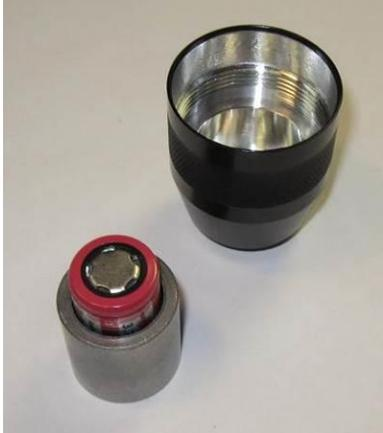
Insert the battery into the spacer
