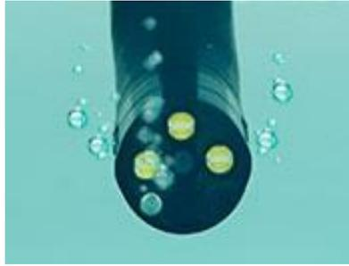
5. Uncover the hole in the Air/Water Reusable Scope Valve and verify that no air bubbles are being emitted from the nozzles.
