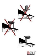
The form of the chimney cap must not obstruct currents of air from the outside. In other words it must allow the air to enter through one side and leave through the opposite side so as not to cause descending currents of air.
