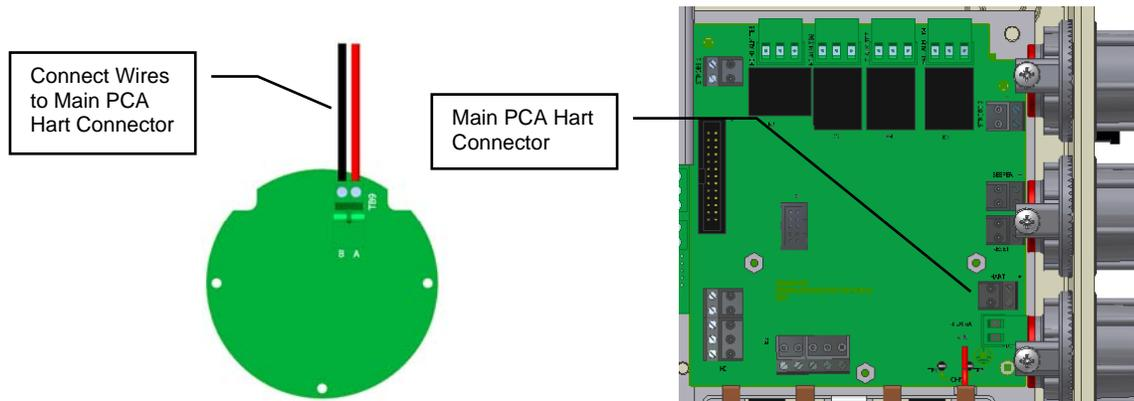
5. Place the HART Card on the Hex Stand-offs and gently couple the Electrical Plug into the jack on the Main Printed Circuit Board Assembly.
