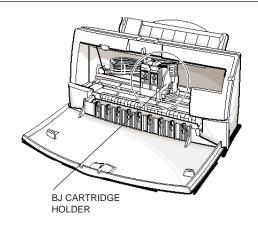
Set the paper thickness lever. O If you installed the BC-20 Black BJ Cartridge, set the paper thickness lever to the left.
