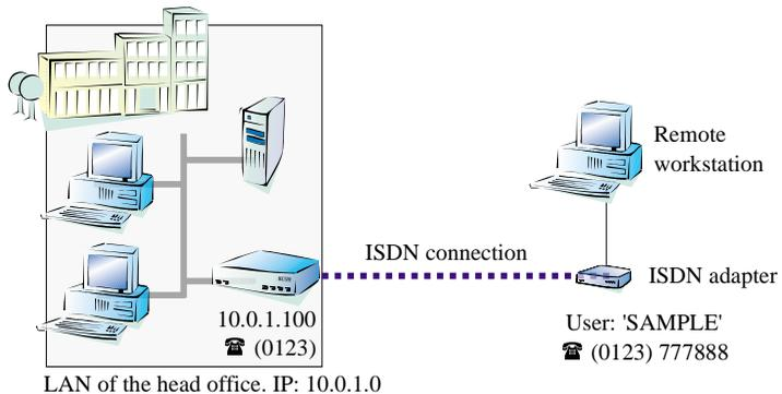
Each active RAS user must be assigned an IP address when using the TCP/IP protocol. This IP address can be permanently assigned when setting up a user. However, it is simpler to let the *Lucent CellPipe 55* automatically assign free IP addresses to users when they dial in. In
