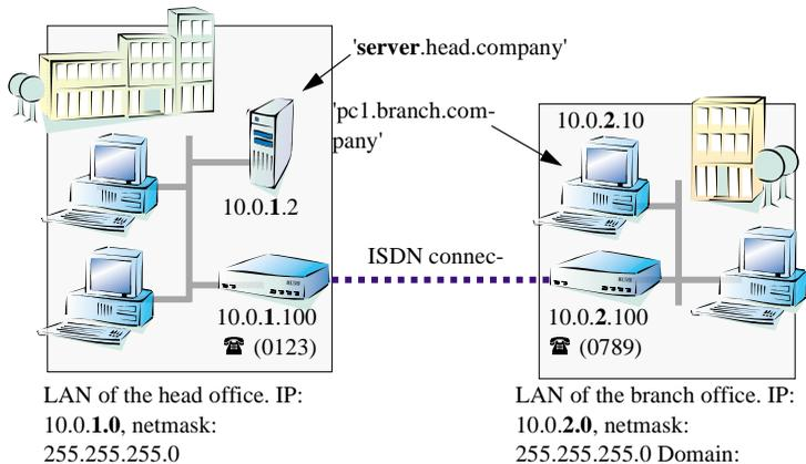
Unlike when accessing the Internet, all of the IP addresses in the involved networks are visible on the remote side when coupling networks, not just those of the router. The computer with the IP address 10.0.2.10 in the branch office LAN sees the server 10.0.1.2 in the headquarters and can access it (assuming it has the appropriate rights), and vice versa.
