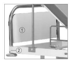
• Insert the head end and leg end bows (1) (fitted with laminated panels) in its brackets (2) at head end and leg end respectively by extending equal forces with both the hands in the bracket as shown above.
