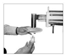
• Fix the rubber buffer in the buffer holder with bush and bolt at all 4 corners as shown above.
