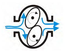
The flow through the meter measurement chamber follows the path of least resistance. Therefore no liquid passes through the center cavity between the rotors. The fluid is displaced from the inlet to the outlet via the area between the smooth oval rotors and the inner diameter of the meter housing.
