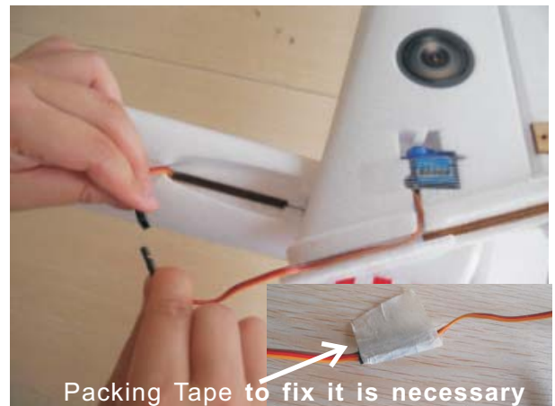
Rudder servo cable connection with Extention cable
