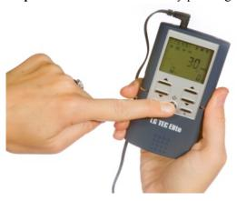
**Step 5:** Press "M" to Select TENS or EMS. Use the "S" button to scroll through the options in your chosen mode. Press the \$\psi\$ arrow down button on either side to select stimulation type.
