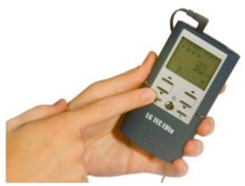
**Step 6:** Select the up arrow on the left until the electrodes connected to that lead wire are strong but comfortable. If using all 4 electrodes, repeat this step using the up arrow on the right side. The amplitude treatment range, or power, is 1-105mA.
