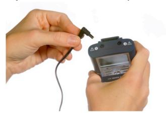
**Step 3**: Connect the lead wires to the electrodes then apply to your body. For TENS mode, use all 4 electrodes in a diagonal pattern over the affected area. For EMS mode, use 2 electrodes over the affected area.
