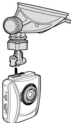
2. With the suction-cup laying flat, position the suction-cup on the windshield.
