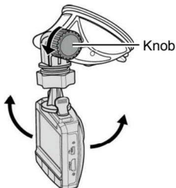
2. Loosen the knob to swivel the device horizontally up to 360°.
