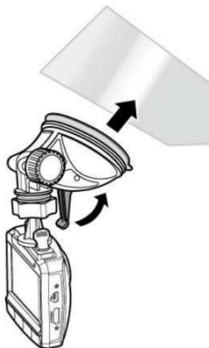
3. Hold the base firmly on the windshield and press down the clamp to mount the car holder to the windshield. Make sure the base is securely locked in place.
