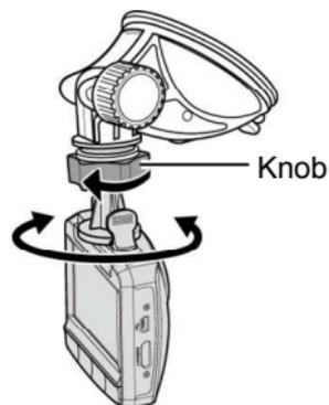
3. Then tighten the knob to make sure the device is securely locked in place.
