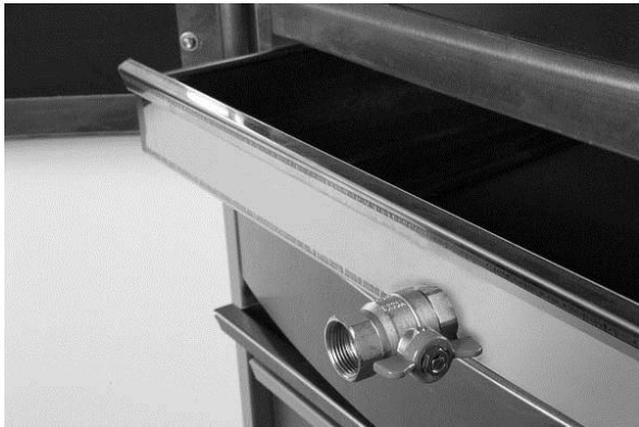
Drain valve open. (Handle horizontally)
