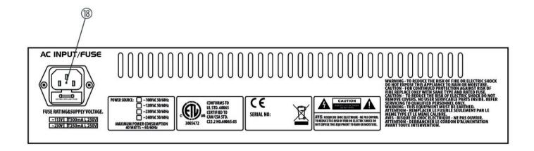
18 IEC chassis connector with fuse holder.
