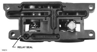
Figure 7-5. Pneumatic Relay Assembly
