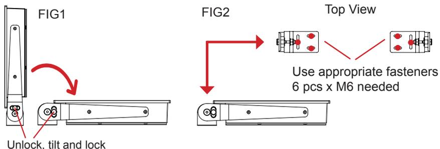
▼ 7: Max Forward and Backward angle shown below (FIG1). When your desired tilting position has been achieved, you need to verify that the Lock Pin are in locking position and the unit is firmly attached and does not appear loose (FIG2).
