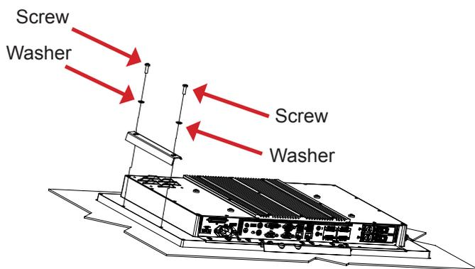
4: Review closeup of the mounting of brackets with screws and C-Washers in place. Seen from bottom side.
