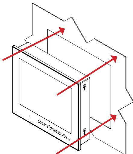
2: Prepare and position the brackets into each of the four key holes. The key part goes into the unit's largest area of the keyhole, while the Allen screw is visible at the top. See closeup.
