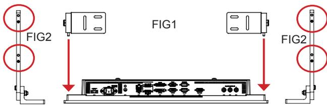
4: While unit is lying flat on table, check the Tilting Lock Pin position. These can be pulled out by hand, turned 90° (FIG1) and turned back 90° until the Lock Pin automatically clicks into place by a spring (FIG2).
