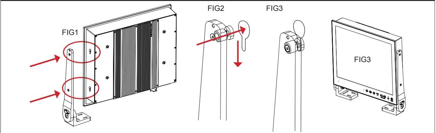
▼ 6: Tighten Key Hole Screw firmly on each side and make sure the brackets are properly mounted and aligned to the main chassis of unit. Verify with your hands that both brackets are firmly attached.
