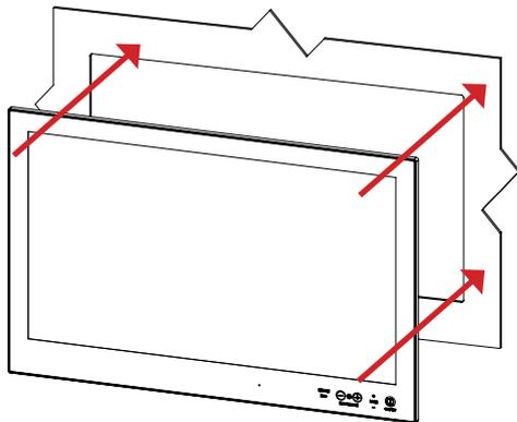
2: Make sure you are aware that brackets should be mounted on TOP, LEFT, RIGHT and BOTTOM sides. Note that the [B] bracket is different than the [A] brackets and mounted near the connectors. See closeup of details.
