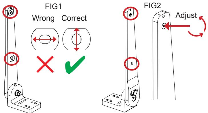
▼ 3: Verify that the Key Hole Set Screw (M4) is aligned with the bracket surface (FIG1). If this screw appear too far out (FIG2), proper fitting into the Key Hole can not be completed. Turn screw clockwise or anti-clockwise (FIG3) to adjust the position.
