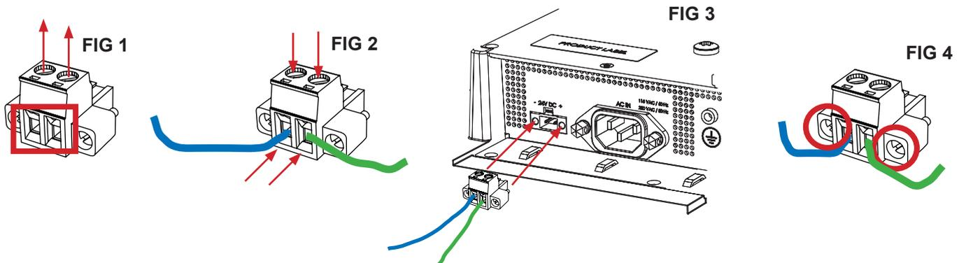
**FIG 1:** Unscrew (from top) or make sure that the screw terminal (square area) are fully open, so you can secure the inserted cables correctly to the loose housing connector (it may already be plugged into the unit as per factory installation).
