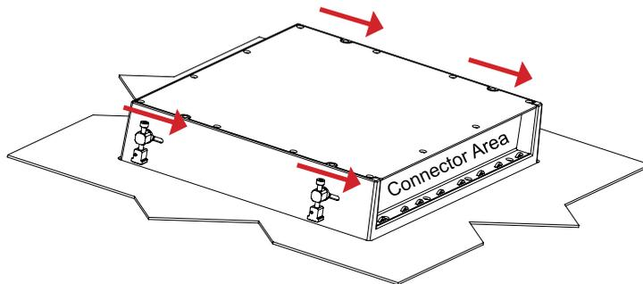
4: Secure the unit by fastening the top Allen screws fairly. Make sure you do it equally and even for all 4 sides. Do not use excessive force. See closeup of a open and closed position to the right.
