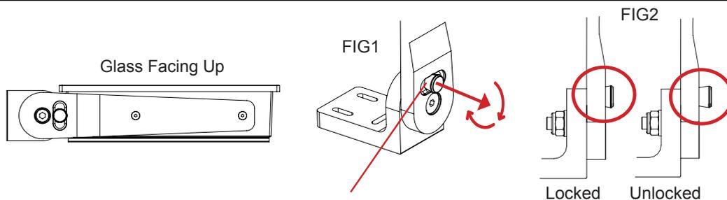
▼ 6: You may now mount the unit onto your desired location. It is advised that you unlock the Lock Pin (as shown in step 5), tilt the unit 90 degrees backwards (FIG1) and properly fasten the bracket base into location (FIG2). **NB! Be careful not to break or scratch the edge of the front glass!**
