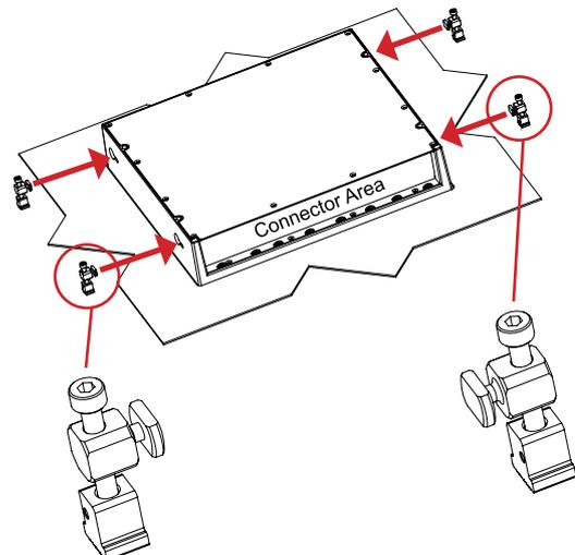
3: When all brackets fits inside the keyhole, slide them down into the narrow gap. If you are unable to slide them down, simply adjust/loosen the top Allen Screw slightly and try again.
