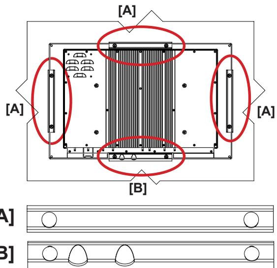
3: Secure each bracket with the provided M5x16 screws and C-Washers as illustrated below. Make sure you do it equally and even for all 4 sides. Do not use excessive force. 2 screws and 2 washers pr. bracket. Note the orientation of brackets before you begin.
