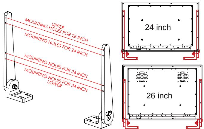
3: Place one bracket at the time with the mounting holes facing down into the suitable mounting position and fasten with 2 x M5 screws on each bracket.
