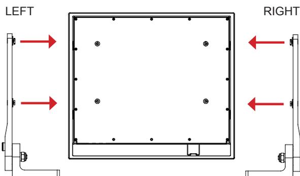
▼ 4: Ensure that both Key Hole Plugs slide into the Key Holes and goes to the upper position (FIG1 and FIG2). If they appear too tight, you may loose the Key Hole Plug screw a few turns and re-try (see previous step 2).
