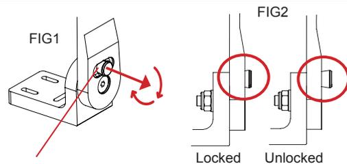
5: You may now mount the unit onto your desired location. It is advised that you unlock the Lock Pin (as shown in step 4), tilt the unit 90° backwards (FIG1) and properly fasten the bracket base into location (FIG2).
