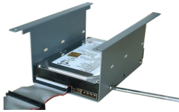
Install the first HD (Master).
