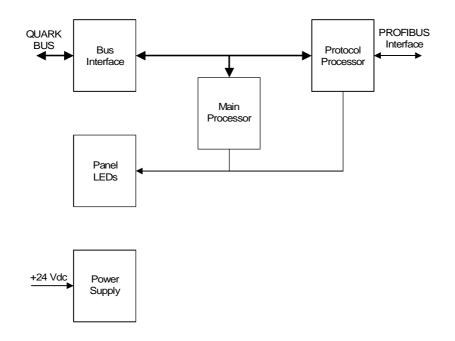
Figure 2-2 Block Diagram of the QK1405
