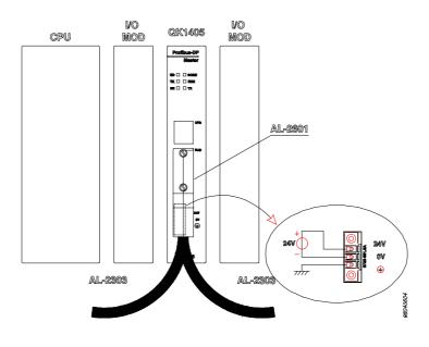
Figure 4-1 QK1405 PROFIBUS Installation
