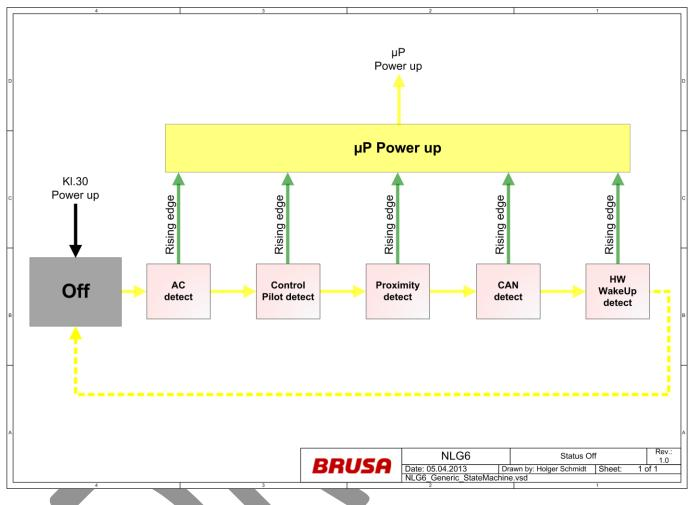
In [State Off], the NLG6 draws only standby current via KL30/31. The hardware monitors the following WakeUp sources:
