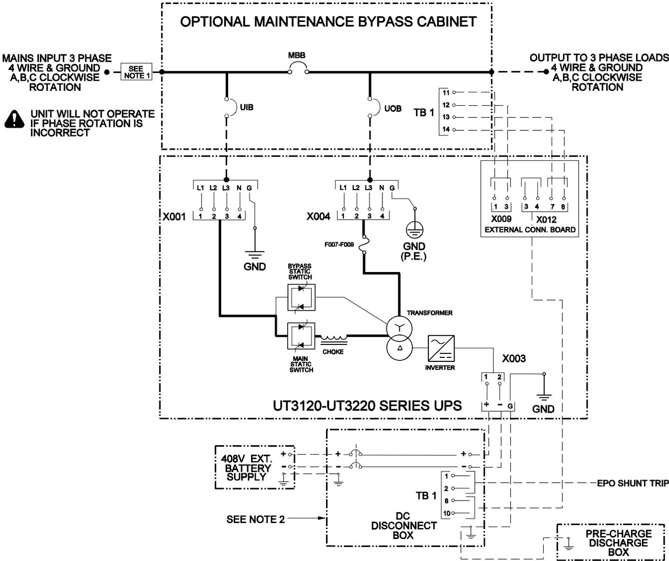
**⚠ UNIT WILL NOT OPERATE IF PHASE ROTATION IS INCORRECT**
