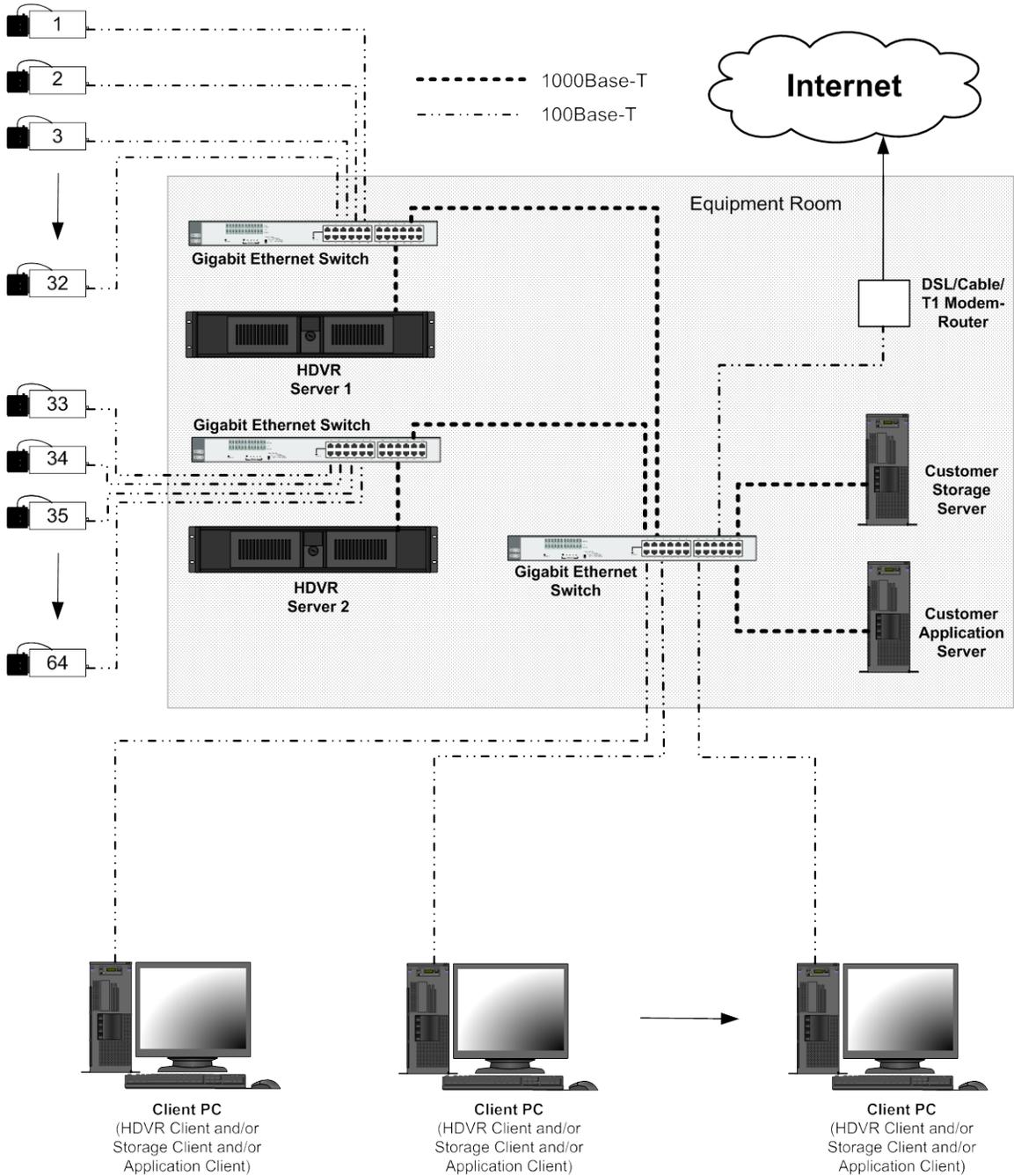
Again, referring to the diagram below, gigabit Ethernet connections are recommended between the HDVR servers and the Ethernet switches, but 100 Mbps connections from the switches to each IP camera and HDVR Client are sufficient.
