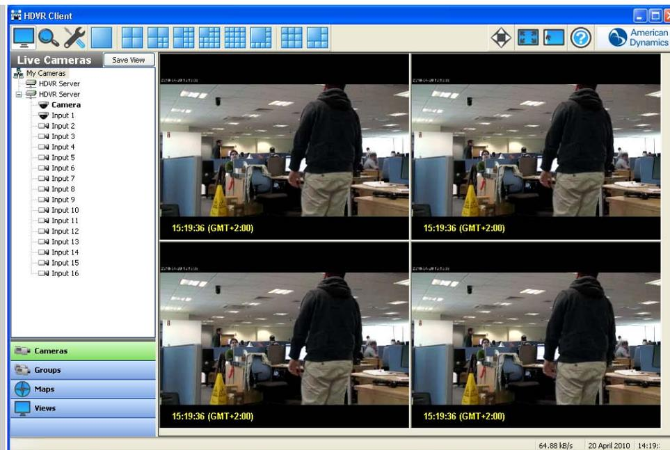
To display live video either drag a camera into the camera display area or click on one of the blue display modes.
