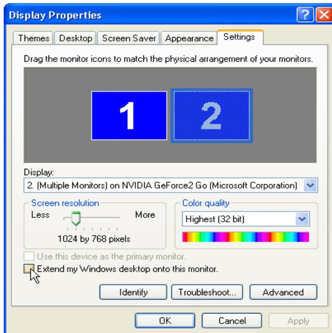
Once you have configured your Windows Display Properties to use multiple monitors, open HDVR client on your primary monitor and drag it to one of your attached monitors. You can then maximize the application to fill the monitor. Return to your primary monitor and open a second HDVR client application. Repeat this process until all of your attached monitors have an open instance of HDVR client.
