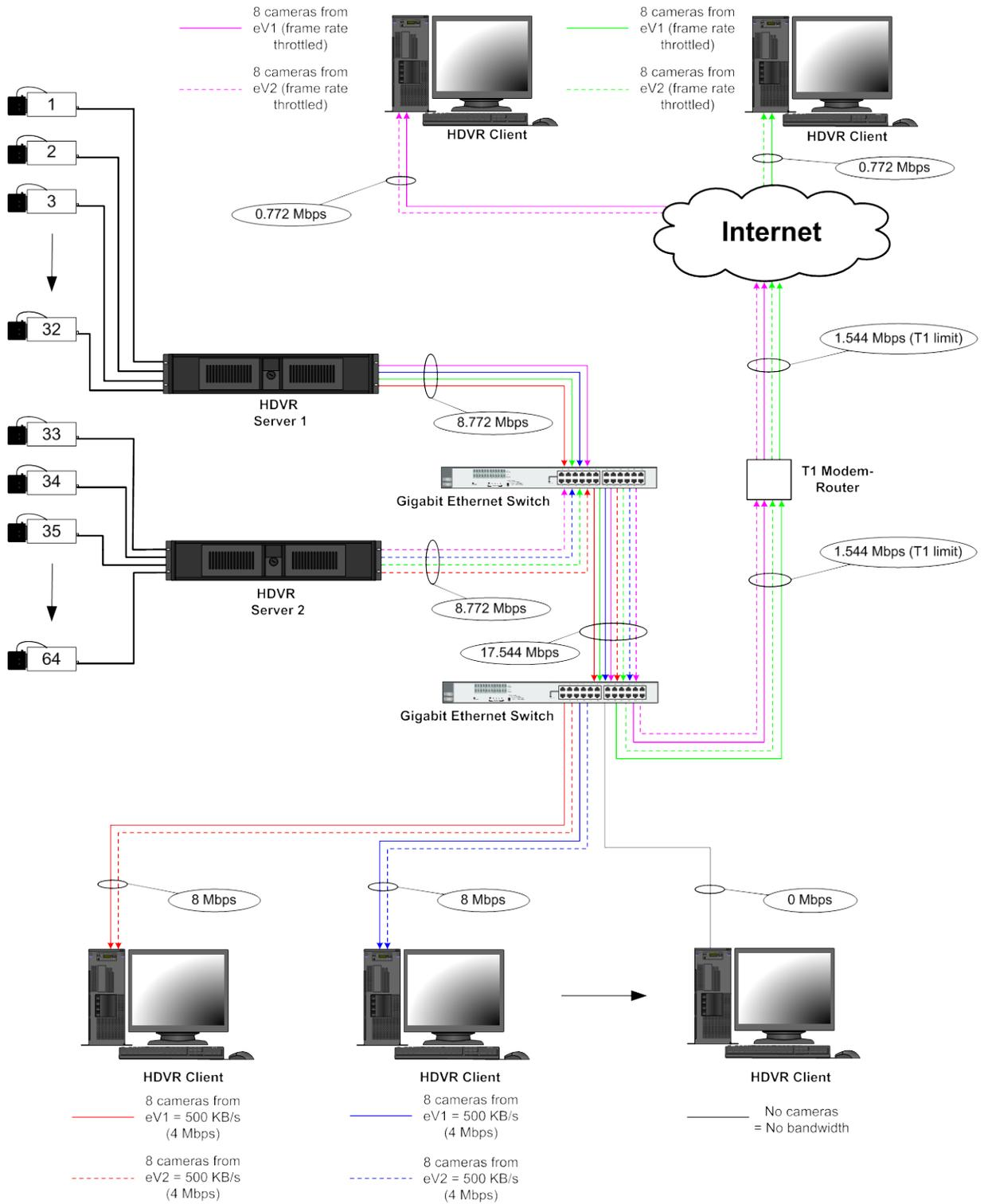
An installation with IP cameras is quite similar. HDVR recommends that the IP cameras are wired in “home-run” style back to an Ethernet switch near the HDVR Server.
