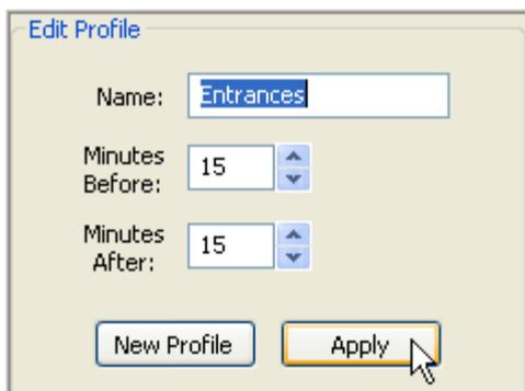
At this point, you have completed the process for creating an HDVR Recall profile, but the system will NOT use your settings until you link the profile to an event on the Event Linking screen.
