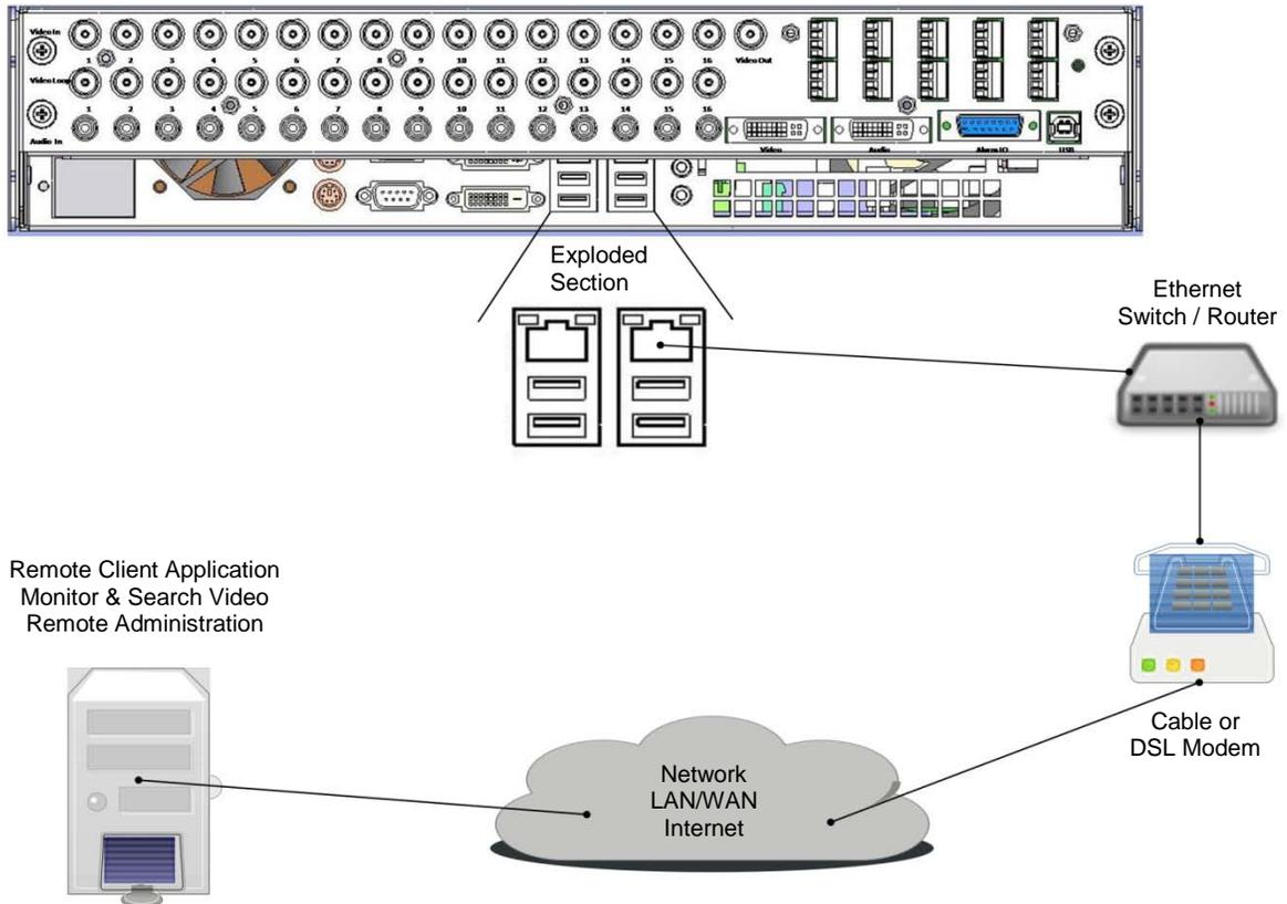
Connect the HDVR 10/100/1000 Mbits/sec Gigabit Ethernet Adapter Port to an Ethernet Switch / Router with Cat5 cable and RJ-45 connectors.
