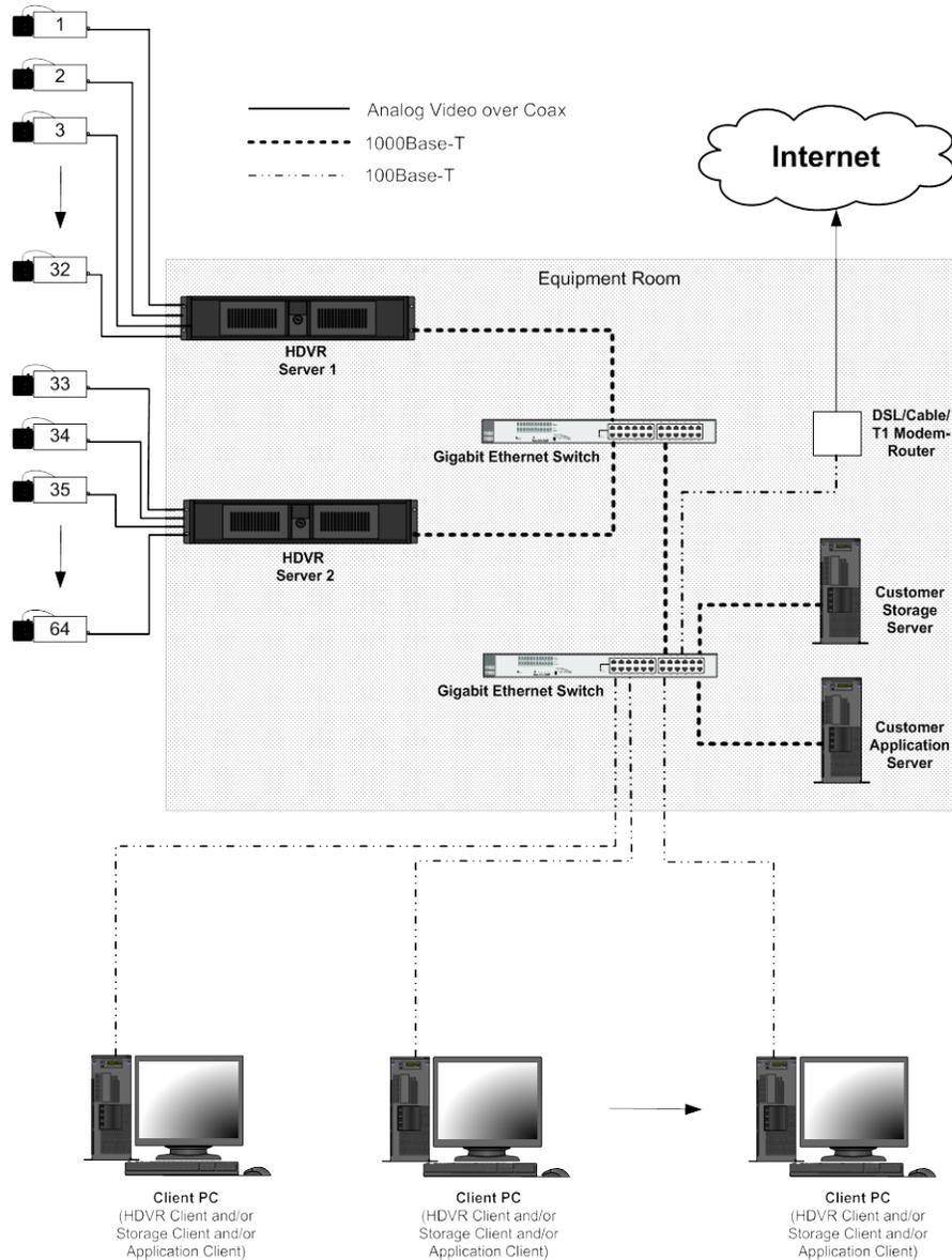
Gigabit Ethernet connections are recommended between the HDVR servers and the Ethernet switch, and between Ethernet switches. While a 100 Mbps connection from the switch to each HDVR Client is sufficient, it can be seen that each active HDVR Client increases the aggregate network bandwidth out of the HDVR server.
