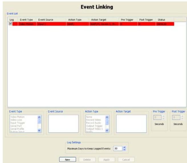
While still on the Event Linking page, locate the “Event Type” box at the bottom of the screen and scroll down to select “Button Input.” Next go to the “Action Type” field and select HDVR Recall. Finally, choose the appropriate profile as the “Action Target.” In this case, we selected “Entrances.”
