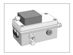
SattTop VB is an electro-pneumatic remote-controlled module. There are two versions, VB1 with one solenoid valve and VB2 with two solenoid valves. Both versions are equipped with the Electronic Unit, SattTop EU.
