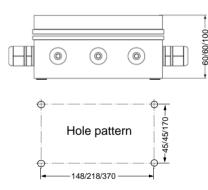
NOTE! The first measure applies for a junction box for 3 valves, the second for a junction box for 6 valves, and the third for a junction box for 20 valves.
