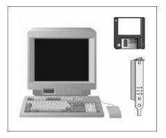
SattTop PCDoc is a configuration and documentation program designed to run on a PC. It is delivered on a 3.5" disk together with a SattBus PC board.
