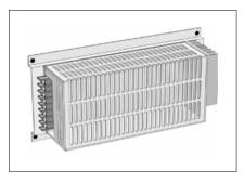
The power supply, SattTop PS2 can supply up to 120 SattTop field units in a loop. Its output voltage (32 V DC) is connected to the trunk cable through a SattTop connection box or a screw terminal.
