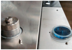
Figure 3-4: Reservoir Fill Port and Sight Glass Lid
