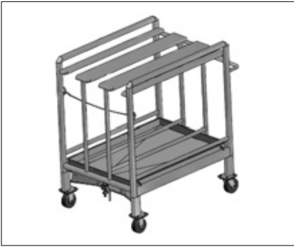
Figure 6-6: Transfer Cart with Safety Cable
