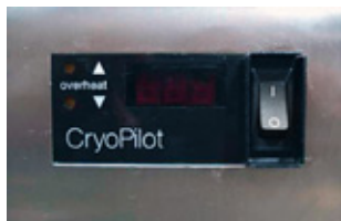
Figure 2-5: Control System Power Switch and Over-Temperature Setting Display
