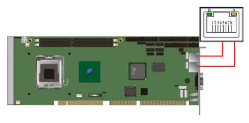
LAN1/LAN2 Link/Active & Speed LED Connectors (CN6, CN7)
