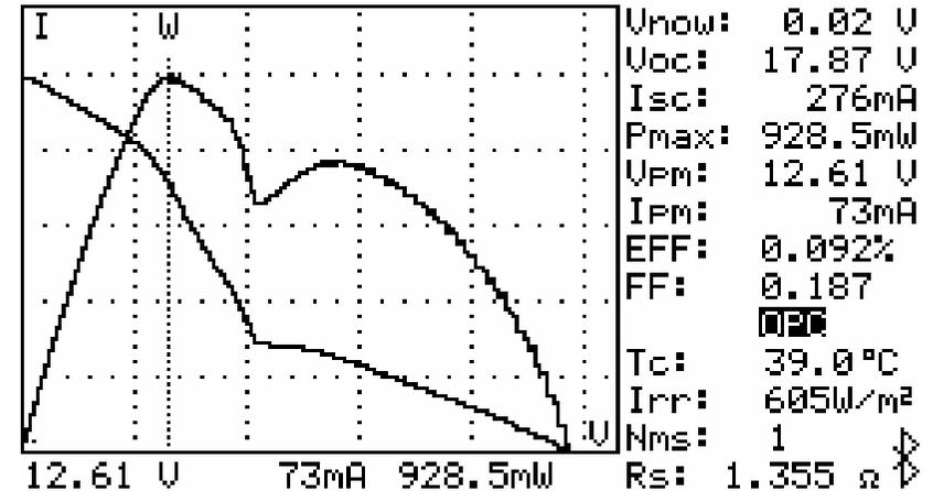
Maintenance engineers can store the characteristics data of solar panels in the beginning. And compare the characteristics data in weekly, monthly or yearly maintenances. If the characteristics of any solar panels are different from the previous data, maintenance engineers can further identify the problems of solar panels.
