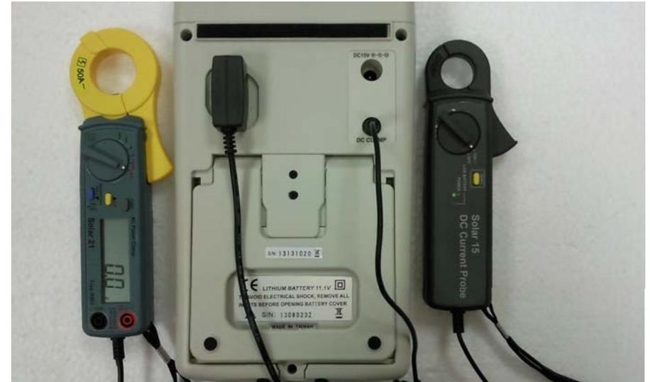
The POWER mode is used to continuously measure/monitor/record the DC power output of solar system and the AC power output of Inverter (1 phase or balanced 3 phases); calculate the efficiency of DC to AC power conversion, the efficiency of the max. output power, DC/AC output power, and Watt/hour, etc.
