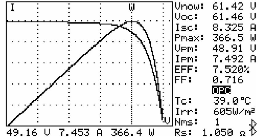
The unit can measure actual max. power (Pmax), voltage (Vpm) and current (Ipm) at max. power. Instead of the rated max. power, system designers need to be aware of the actual solar power from solar panels under actual operating conditions. So designers can actually know how many pieces of solar panels are required to generate specific power.
