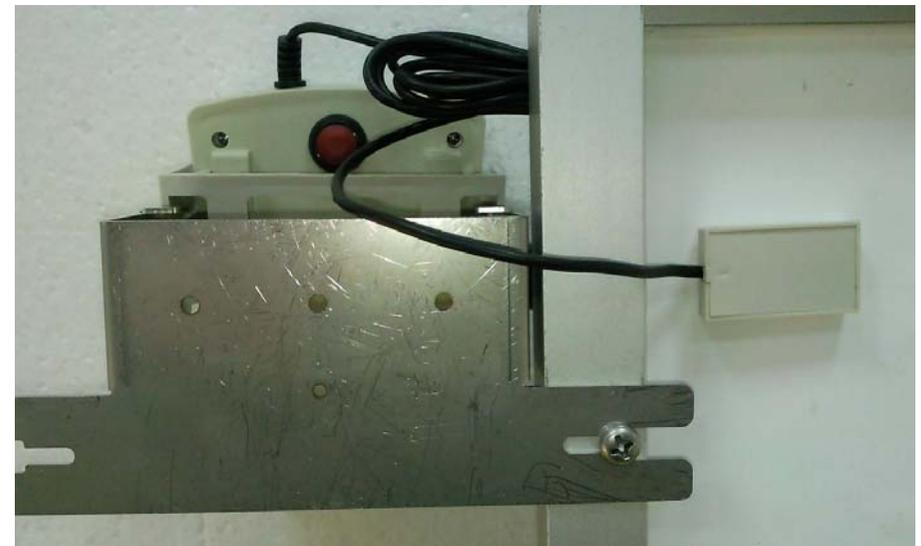
Use Thermal conductive gel to stick Auxiliary thermometer on the Solar panel (back side)
