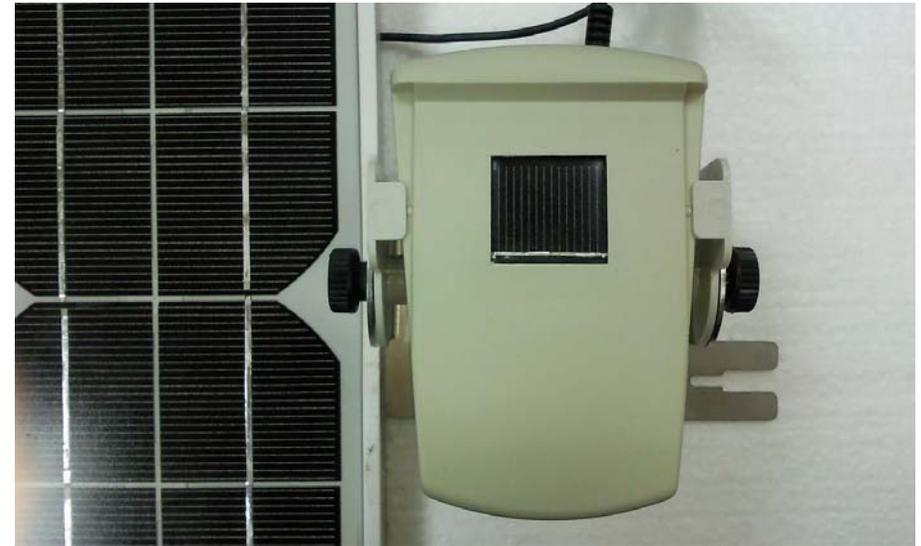
Connect the Solar panel (front side) with Remote solar detector
